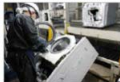
Drum-type washing machine disassembling line
